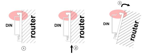
Figure 14: Removal of the DIN Rail
