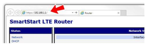
Figure 25: Entering the IP address of the router
