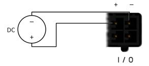
Figure 17: Connection of power supply
