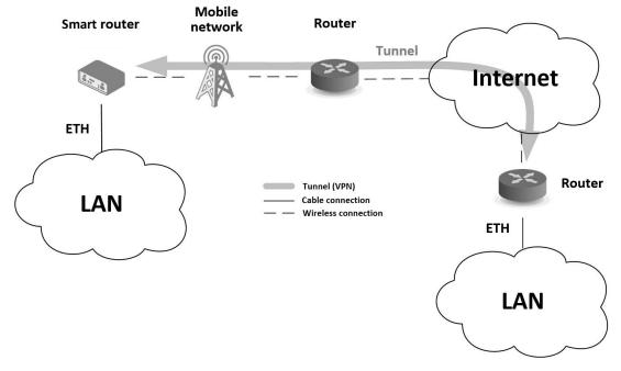
Figure 3: Using a VPN tunnel
