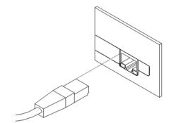
Figure 21: Connection of Ethernet cable
