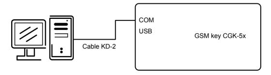
• cable KD2 is connected to PC serial port (example COM1)
